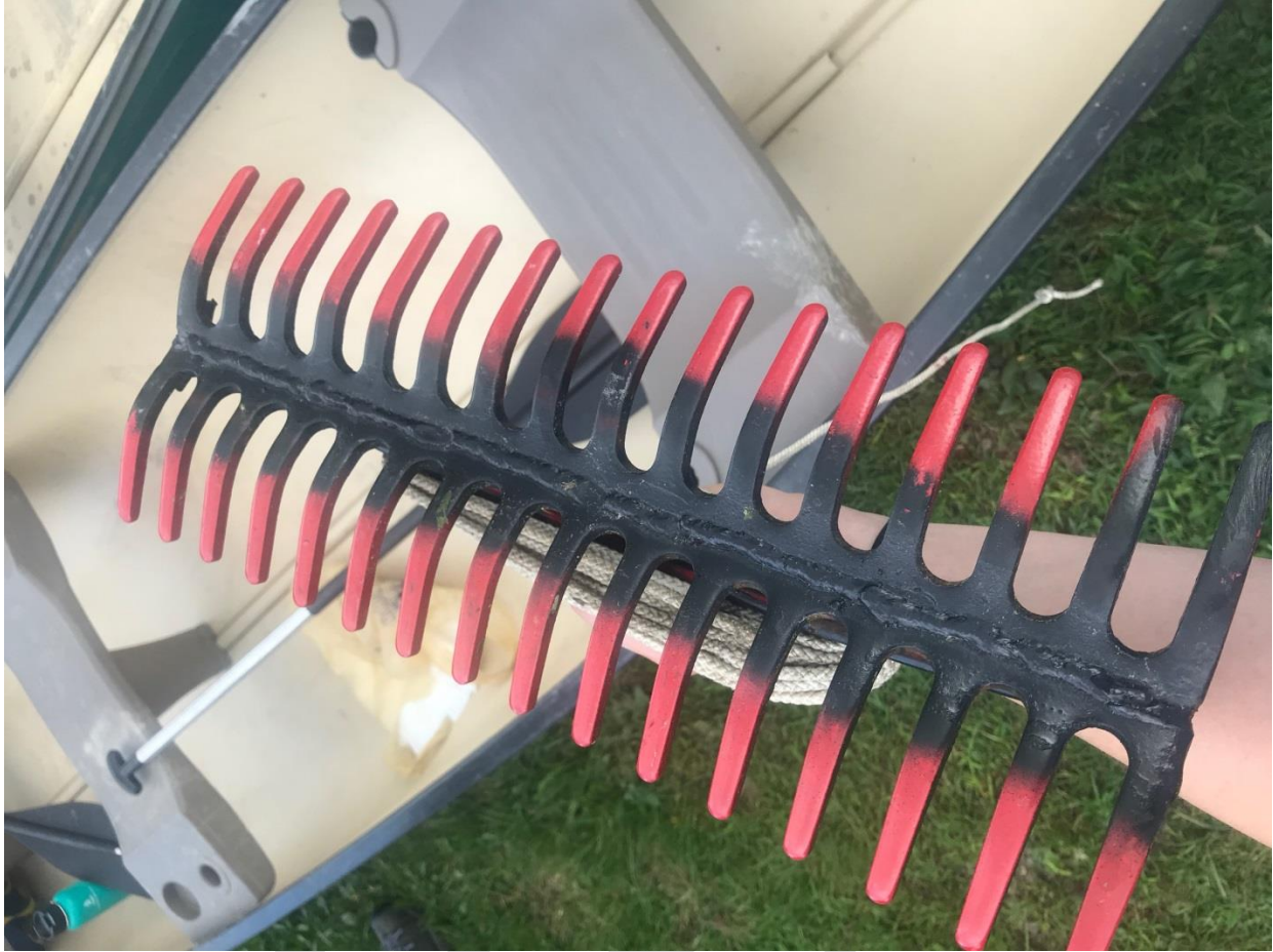
Fig 6 Plant rake used to collect macrophytes. Line is attached to a point on the watercraft, and rake is tossed into the water. Once the rake has hit the sediment, is it retrieved into the boat and macrophytes collected are observed.
